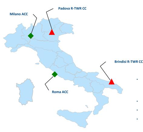
2 ACC  2 ACC, one in Rome and one in Milan, to manage en-route traffic; integration in 2 ACCs of approach radars currently in towers
