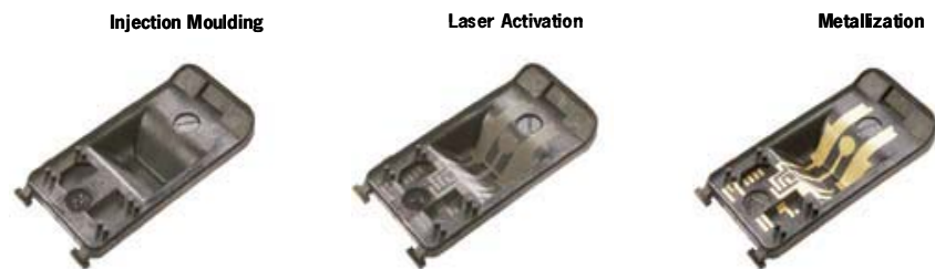
Fig 6 The LPKF-LDS process
